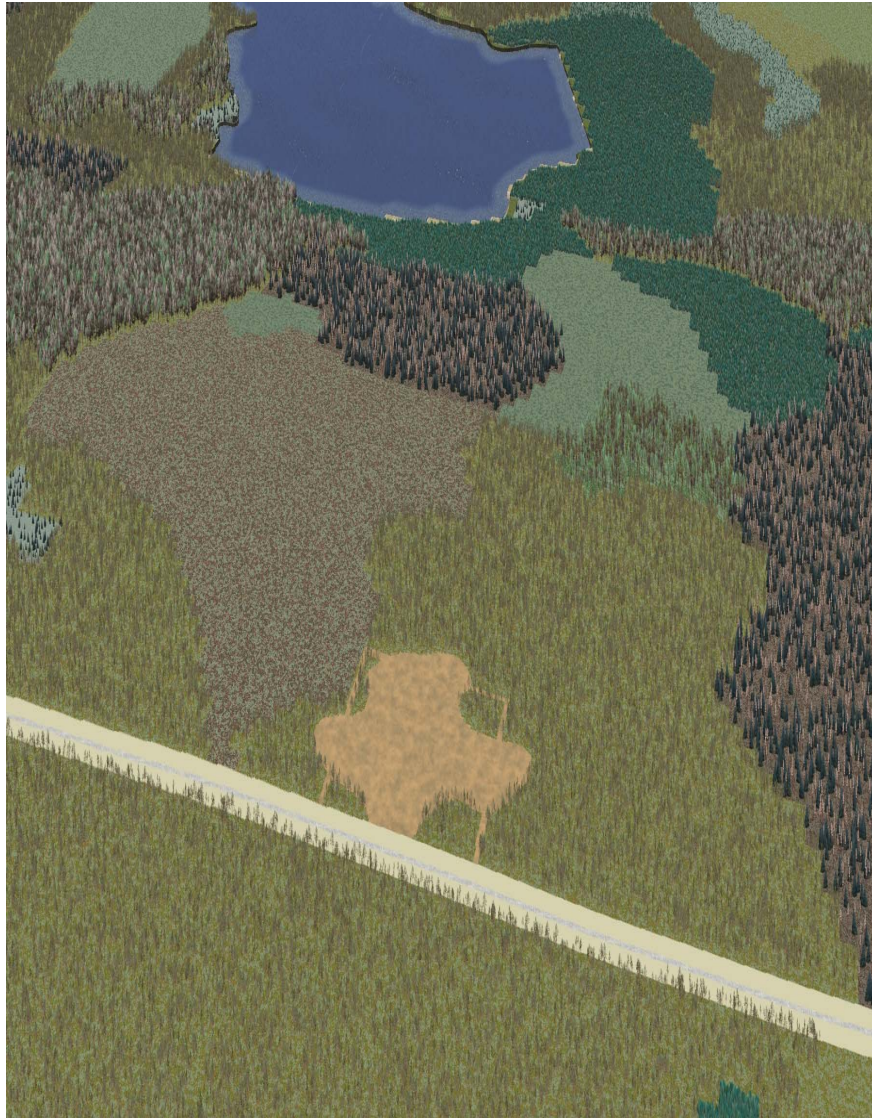
Figure 4 - Organic shaped drill site compared with traditional square. When organic shapes are used the total area disturbed is normally larger than for square or rectangular sites due to safety requirements.
