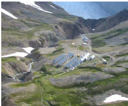
Camp for a large MX project. Camp access was via air transport and given the elevation, care was taken to construct the camp to withstand snow loading.
