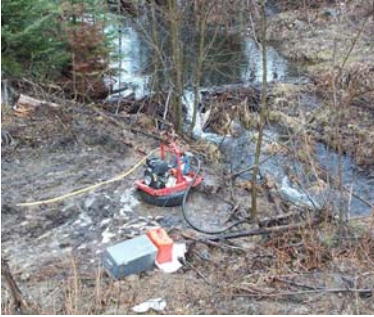
Streamside water supply pump - the pump and motor are seated in a containment tray and the ground is buffered by a tire.
