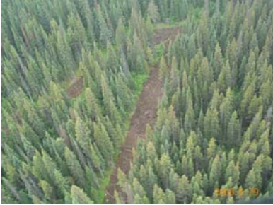
Reclamation on a trail with a 10-m right-of-way. Soil and debris have been pulled back onto the trail and are ready to be replanted.
